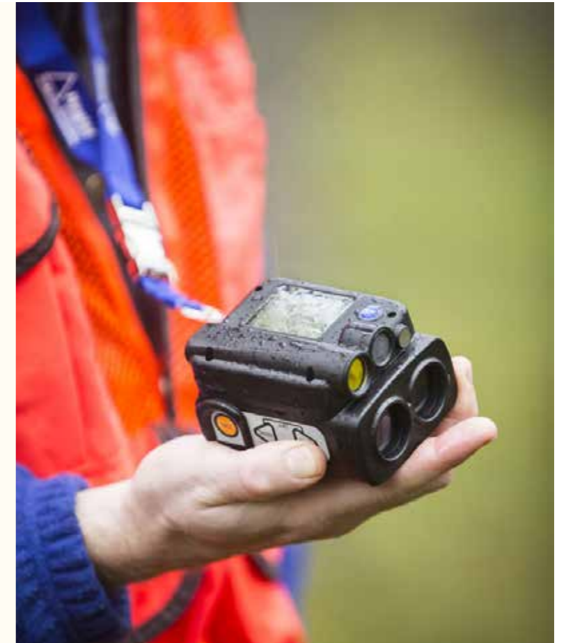
Haglöf's Vertex Laser instrument VL5 is a unique combination instrument featuring both ultrasound and laser technology with very high accuracy and many built-in applications that offer operators in forestry, utility industry and construction areas high versatility and reliable precision measurement.
