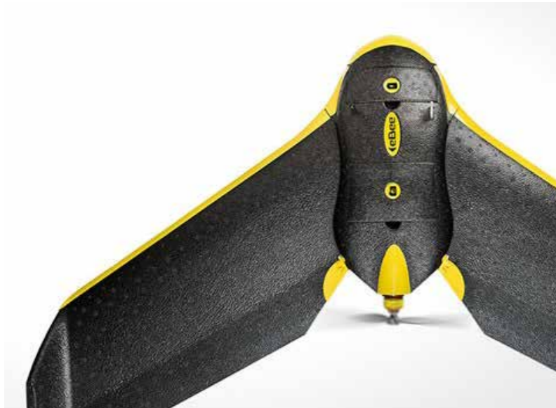
The eBee uses a rear-mounted propeller and due to its flexible foam construction it weighs 700 g (1.5 lbs), minimizing its impact energy.
